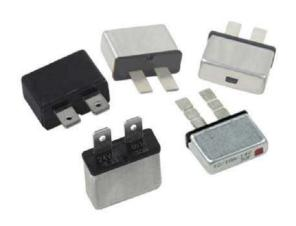
E31 is a single pole,snap-action, automatic reset (SAE Type  $\,\mathrm{I}\,$ ) circuit breaker designed to protect wiring harnesses, battery powered riding toys , portable power tools and many other applications with operating voltage up to 24 Volts DC or 240 Volts AC . Provides a compact profile , broad design flexibility and versatile mounting options . E32 is modified reset (SAE Type  $\,\mathrm{II}\,$ )
